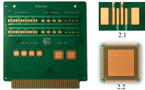
Figure 2. Custom-designed SIR board under Passives/QFNs
